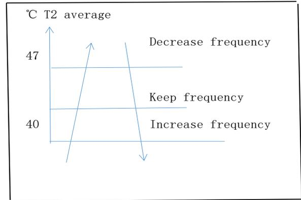
**Use the following table and final capacity request to confirm the operating frequency.**
