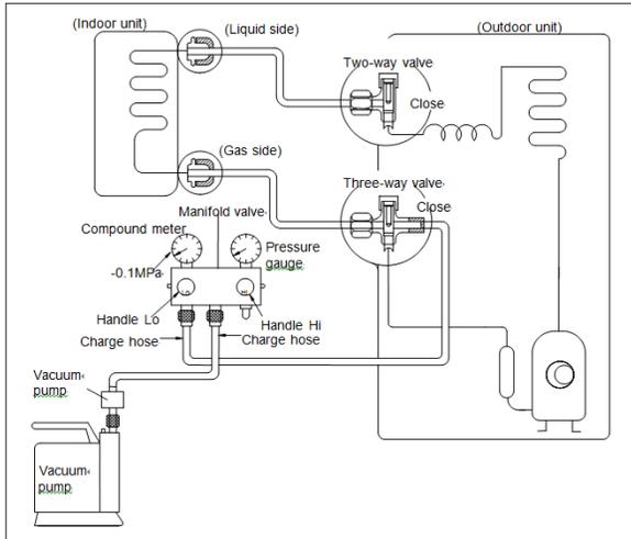
1. Completely tighten the flare nuts on the indoor and outdoor units. Confirm that both the 2-way and 3-way valves are set to the closed position.
