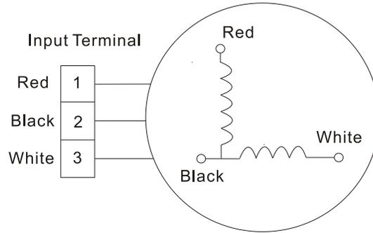
2. Indoor DC fan motor (control chip is inside fan motor)
